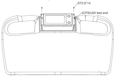
3. Attach the outer frame panel to the bed end.
